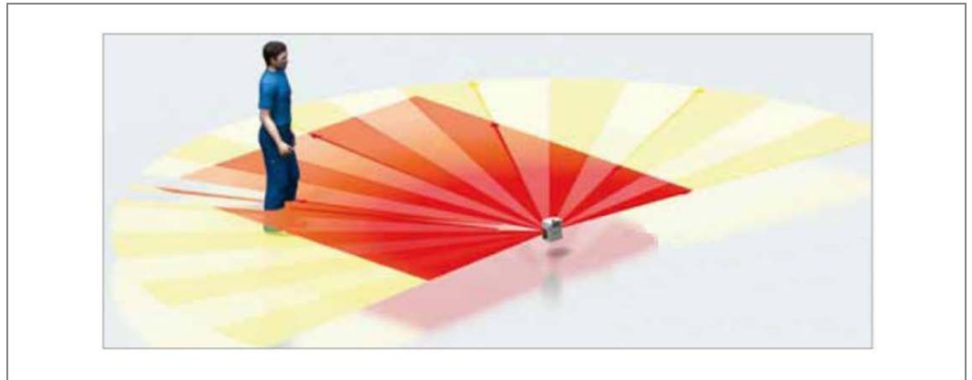
Fig. 1: 2D laser detector principle of operation
