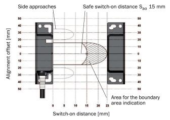
If the actuator moves laterally in relation to the surface of the sensor, a minimum distance of 9 mm must be maintained. This distance will prevent premature triggering due to the side approach areas.
