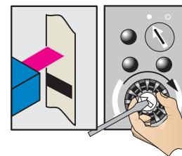
Turn the potentiometer forward again by half the number of turns to ensure that the switching threshold is optimally set.
