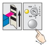
Release the teach-in button. Yellow LED will illuminate, when emitted light is on the mark.
